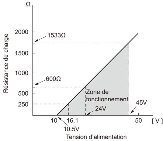
Note: For communication with HHC<sup>(1)</sup> (Model: FXW), min. of 250 W required.
